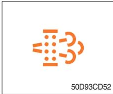
① This lamp lights ON when the SCR cleaning is needed and lamp flashes when manual SCR cleaning is activated as table below.
